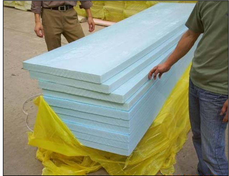
Pictured: Rigid insulation helps insulate the building and lowers the energy demand for heating and cooling the library.
